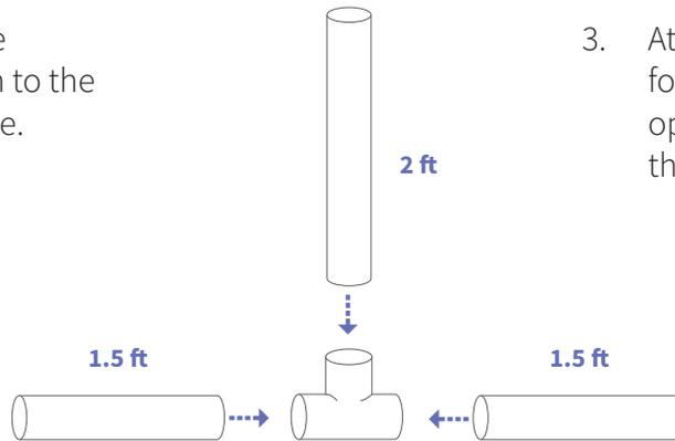
3. Attach the two 1.5-foot sections into opposite ends of the T-junction.
